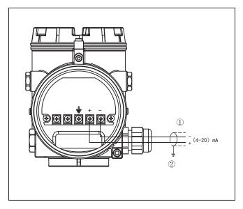
Electronics and terminal compartment, double chamber housing
